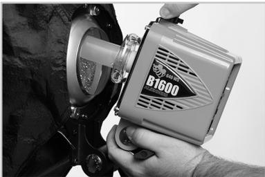
**Mount your flash unit to the softbox.** With your flash unit powered OFF and unplugged, attach it to the SBA adapter and speedring as you would attach any traditional softbox speedring or reflector, using the faceplate quick-release lever (or antennae, on AlienBees units) to expand and contract the faceplate holding fingers. Contract the four fingers, place them inside the SBA center hole, then release the lever/antennae to expand the fingers and hold the position secure.
