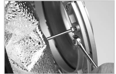
**Loosen the hexagonal metal nuts on the softbox frame poles.** Using the **provided 7mm wrench** (included with each SBA adapter), twist left to loosen the nut on each of the four softbox frame poles.
