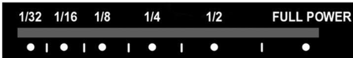
The flashpower is adjusted with a slider on the unit's back control panel.
