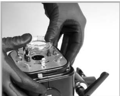
Installing the new flashtube
