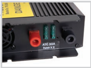
Fuses (on bottom of inverter)
