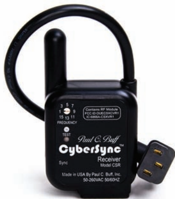
CSR AC-powered (50VAC to 260VAC, 50/60HZ)
